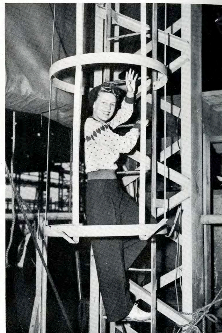
"See you all at lunch," says Lois, as she climbs the 30-foot steel ladder to her overhead crane. The crane travels the length of the bays in the prefabrication building carrying steel from the Plate shop to Assembly.
